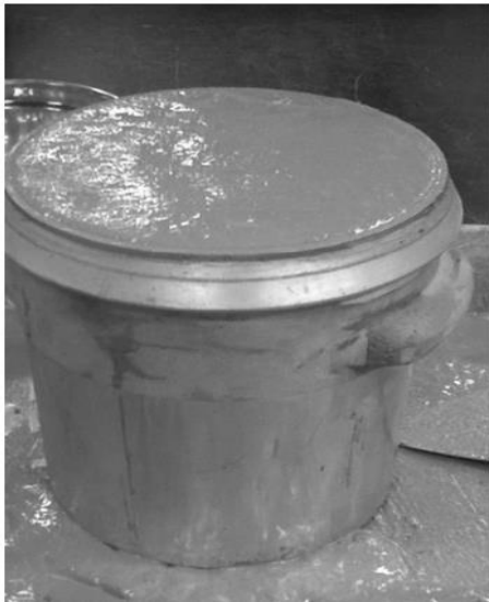
Figure 12 Unit Weight Testing of Concrete
