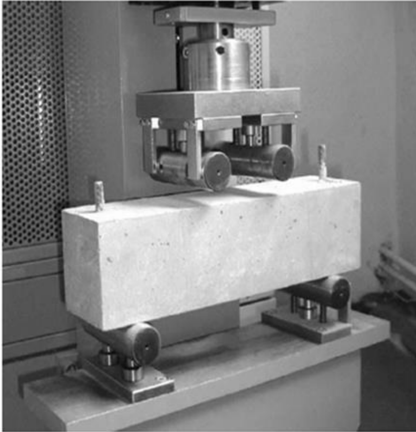
Figure 6 Concrete Modulus of Rupture Testing applying a Third-Point Loading
